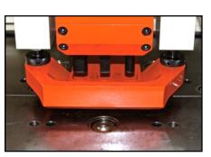
Optional Triple Punch Attachment Fully integrated and pneumatically controlled via CNC Control for increased versatility!
