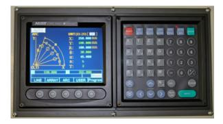
HUST H4N Controller - Upgrade Large Color Screen Control. USB Storage Interface for unlimited Program storage. Ultra-reliable PLC; dust-free design.
