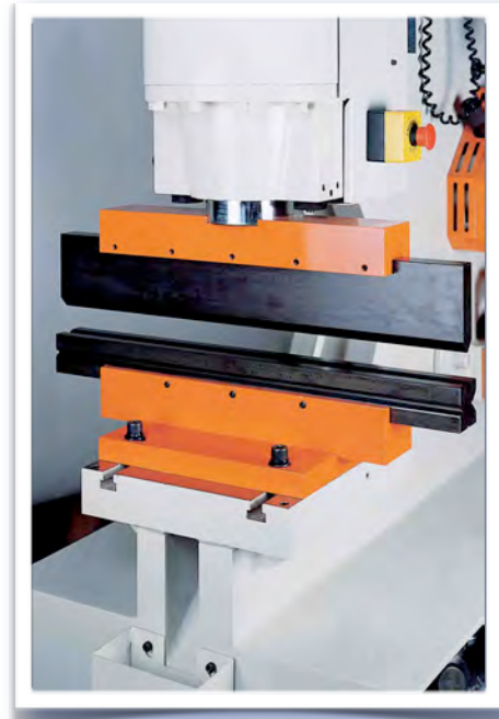
Press Brake Attachment Multi (V) 4-way lower die (3/8", 7/16", 5/8", 15/16")
